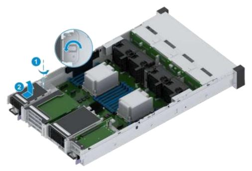
Figure 3-39 Removing the Hard Disk Cage of I/O Module 2 or 3
