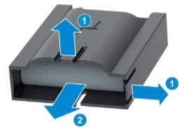
7. Put the removed super capacitor into an antistatic packing bag and record the bar code of the super capacitor.
