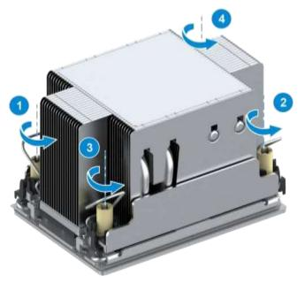
6. Pull the anti-tilt latches in the following directions to unlock the heat sink, see Figure 3-76.
