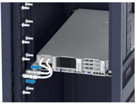
4. Use hook-and-loop fasteners to bind the liquid cooling pipes and connectors.
