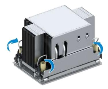
7. Slowly take out the CPU heat sink in vertical direction, turn it upside down, and place the CPU heat sink on the antistatic table, see Figure 3-77.
