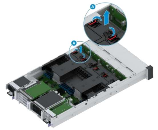
5. Put the removed fan unit into an antistatic packing bag and record the bar code of the fan unit.
