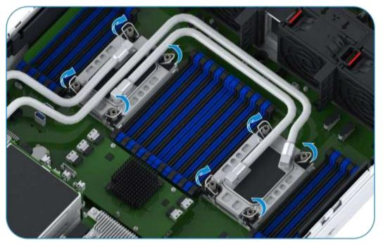
9. Push the liquid cooling panel in the direction of the arrow until it reaches the stop, and lift the liquid cooling panel and two liquid cold plates, see Figure 3-82.
