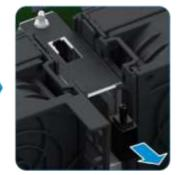
6. Record the bar code of the removed anti-intrusion sensor and put it into an anti-static bag.
