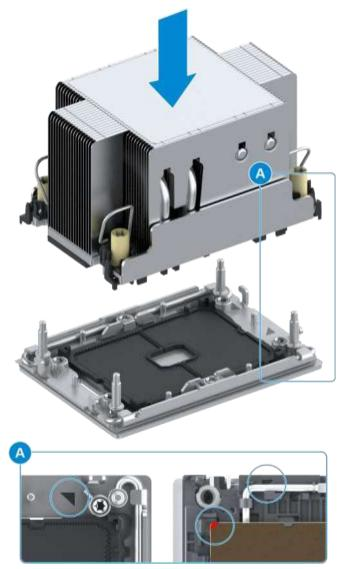
9. Pull the anti-tilt latches in the following directions to lock the heat sink, see Figure 3-90.
