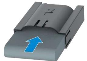
5. Align the three fixing posts at the bottom of the super capacitor box to the three jacks on the air baffle, and install the super capacitor box on the air baffle in the direction of the arrow until the latch of the super capacitor box locks the air baffle, see Figure 3-68.
