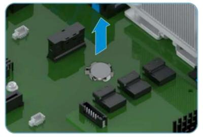
6. Put the removed mainboard battery into an antistatic packing bag and record the bar code of the mainboard battery.
