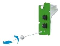
7. Put the removed left flange into an antistatic packing bag and record the bar code of the left flange backplane.
