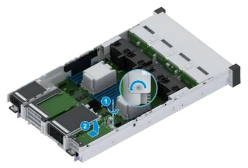
Figure 3-48 Removing the I/O module Bracket 2 or 3
