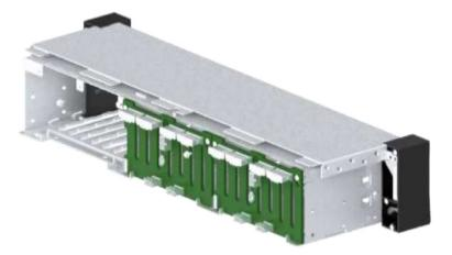
• Backplane supporting 24 hard disks, which is composed of three backplanes of 8 front hard disks, see Figure 3-31.
