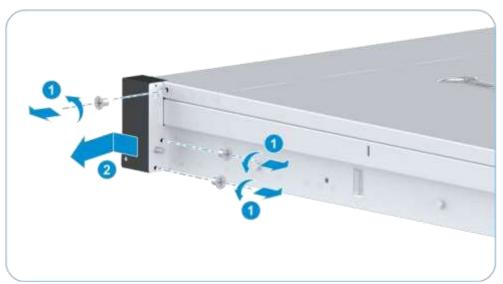
4. Push the right flange towards the front of the server until it cannot be moved, and slowly remove the right flange to the outside of the server, as indicated by (2) in Figure 3-118.
