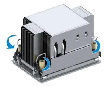
10. Use a T30 Torx screwdriver to tighten the four screws used to fasten the CPU heat sink by following the sequence marked on the heat sink, see Figure 3-91.
