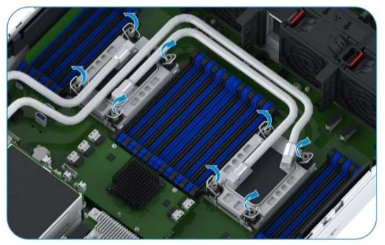
12. Use a T30 Torx screwdriver to tighten the eight screws used to secure the liquid cold plates by following the sequence marked in the figure, as indicated by (2) through (4) in Figure 3-99.
