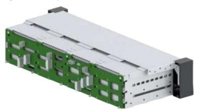
Backplane supporting 16 hard disks, which is composed of two backplanes of 8 front hard disks, see Figure 3-30.
