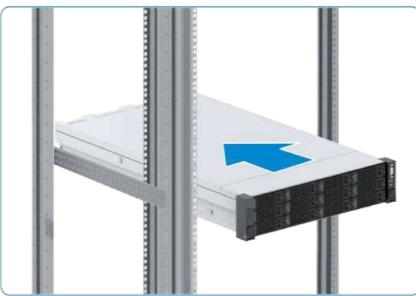
3. Open the screw shielding covers under the front panel of the 2230-RE server, and secure the server onto the cabinet with screws, see Figure 2-13.
