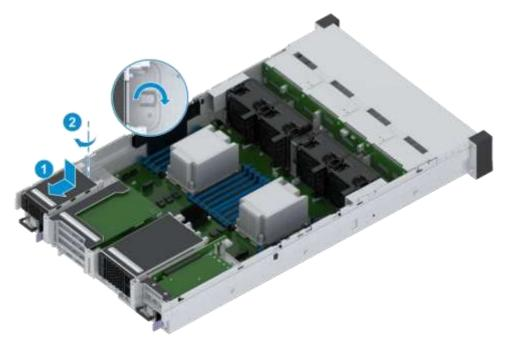
Figure 3-41 Installing the Hard Disk Cage of I/O Module 2 or 3
