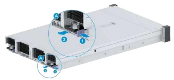
8. Put the removed power module into an antistatic packing bag and record the bar code of the power module.
