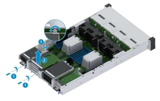
Removing the PCIe Card
