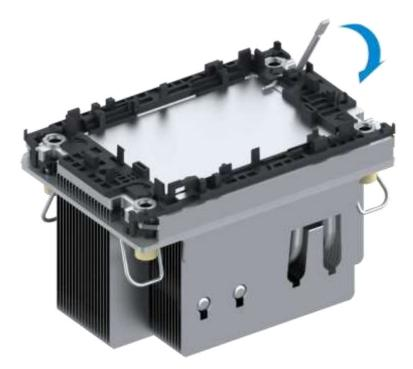
7. Align the corner of the CPU with a triangle mark with the triangle mark on the CPU bracket, place the CPU vertically in the CPU bracket, and gently press the sides of the CPU so that the clips on the CPU bracket are locked to the edges of the CPU, see Figure 3-88.
