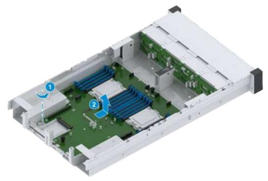
16. Hold the two handles on the mainboard, and slowly push the mainboard in the direction indicated by the arrow until it cannot be moved, and remove the mainboard, as indicated by (2) in Figure 3-106.
