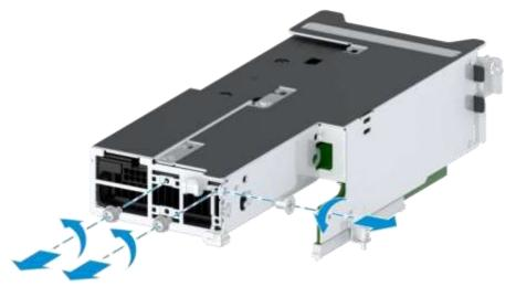
8. Remove the GPU support bracket in the direction of the arrow, see Figure 3-55.
