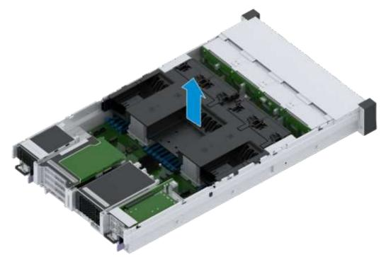
6. Put the removed air baffle into an antistatic packing bag and record the bar code of the air baffle.
