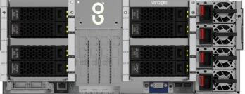
Vantageo 4440-RE is a new-generation 4U 4 -socket compute intensive rack server, which supports 4 Intel ® Xeon ® 4th generation scalable processor (Sapphire Rapids) Vantageo 4440-RE uses a high-density, modular, and streamline design. It features high capability, large capacity, high reliability, easy expansion, and easy management, which is widely applicable to large sacle databases, High Performance Computing, cloud, big data, CRM, ERP and virtualization
