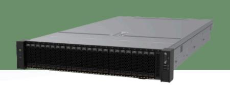
Vantageo 2240-RE is a new-generation 2U 2-socket general rack server, which supports 2 Intel ® Xeon ® 4/5 generation scalable processor (Eagle Stream). Vantageo 2240-RE uses a high-density, modular, and streamline design. It features high capability, large capacity, high reliability, easy expansion, and easy management, which is widely applicable to interconnection, network, cloud computing, big data, and virtualization.
