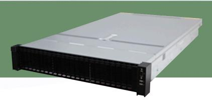
Vantageo 2230-RE is a new generation 2U 2-Socket general rack server developed by Vantageo, supporting two Intel ®Xeon ® third generation extensible processors (Ice Lake). Vantageo 2230-RE is designed with high density, modularization and streamline. It features high performance, high reliability, easy scalability and easy management, which is widely applicable to Internet, cloud computing, big data and NFV.
