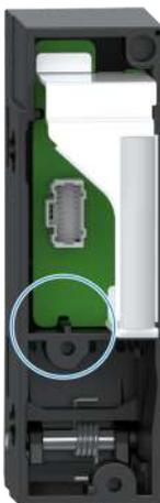
6. Lock the large hole of the gourd-shaped hole on the left flange into the T-shaped stud on the left of the server, and push the left flange to the rear of the server until it reaches the stop, see © in [Figure 3-108](#).
