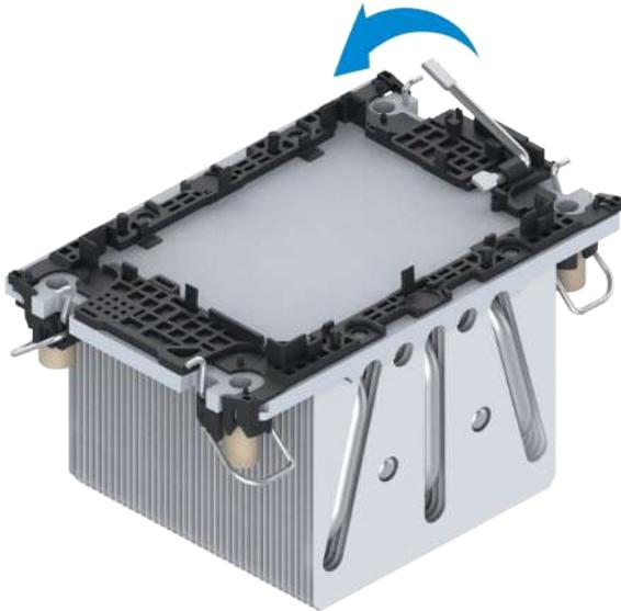
6. Align the corner of the CPU with a triangle mark with the triangle mark on the CPU bracket, place the CPU vertically into the CPU bracket, and gently press the sides of the CPU so that the clips on the CPU bracket are locked to the edges of the CPU, see [Figure 3-88](#).
