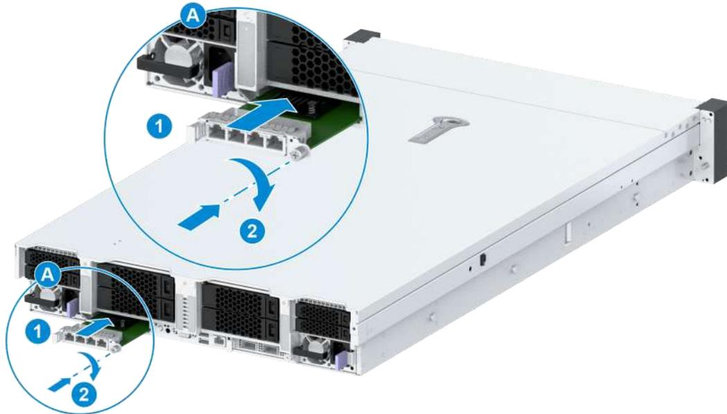
4. Tighten the captive screw of the OCP card by using a PH2 crosshead screwdriver, see ② in [Figure 3-12](#).
