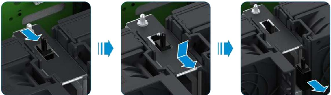
6. Record the bar code of the removed anti-intrusion sensor and put it into an anti-static bag.
