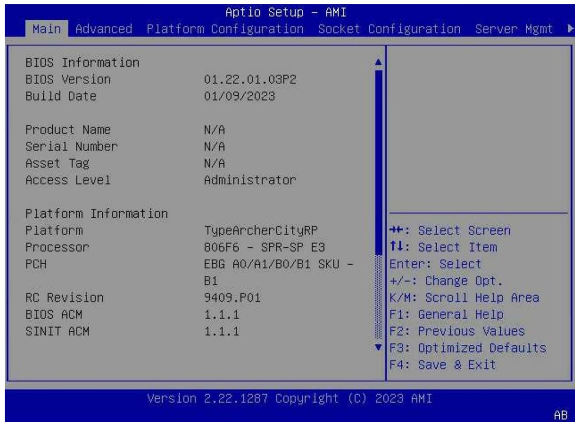
8. On the **Setup** screen, select the **Main** menu. The **Main** screen is displayed.
