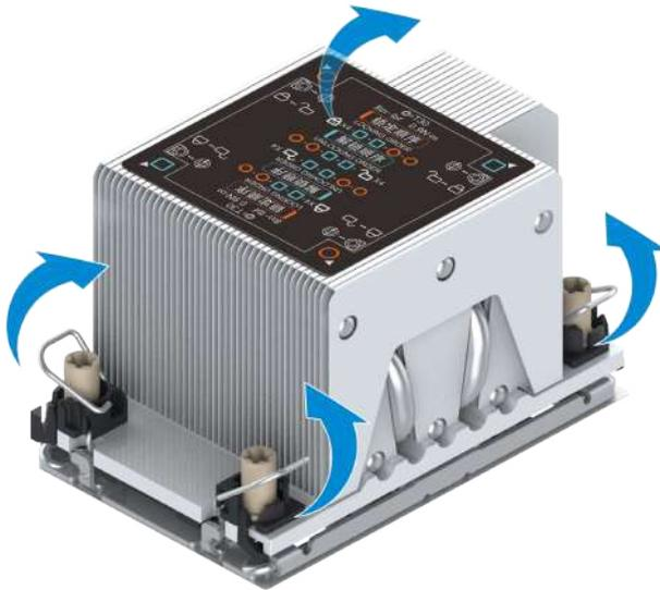
8. Slowly take out the CPU heat sink in vertical direction, turn it upside down, and place the CPU heat sink on an anti-static table, see [Figure 3-84](#).
