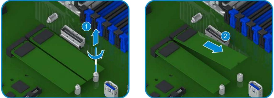
5. Lift the rear end of the M.2 SSD to an angle of 20 to 30 degrees above the horizontal line and pull the M.2 SSD out in the arrow direction, as indicated by ② in [Figure 3-69](#).
