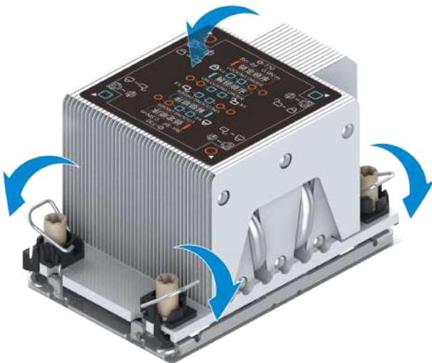
9. Use a T30 Torx screwdriver to tighten the screws used to fasten the CPU heat sink by following the sequence marked on the heat sink.
