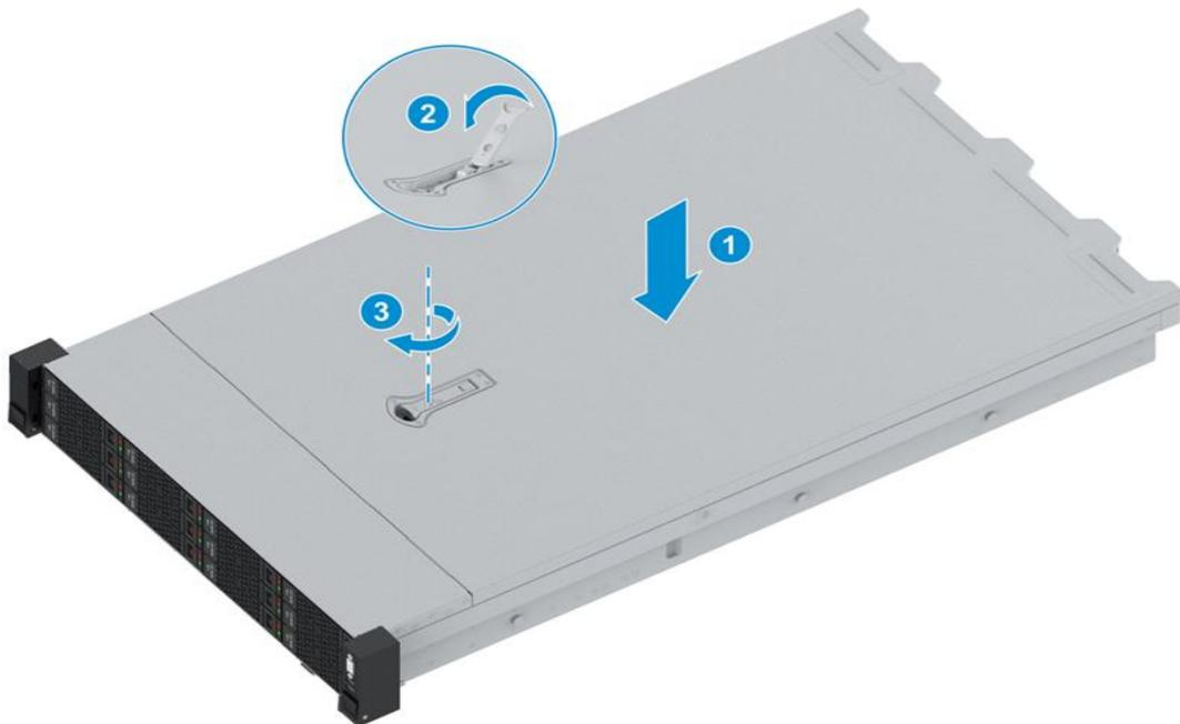
4. Close the ejector lever of the server cover and install the cover, see ② in [Figure 2-12](#).
