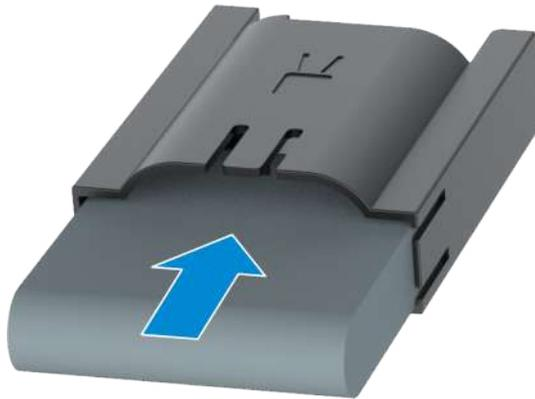
4. Align the three fixing studs at the bottom of the supercapacitor box with the three holes on the air baffle, and install the supercapacitor box on the air baffle in the direction of the arrow until the latches of the supercapacitor box lock the jacks of the air baffle, see [Figure 3-74](#).
