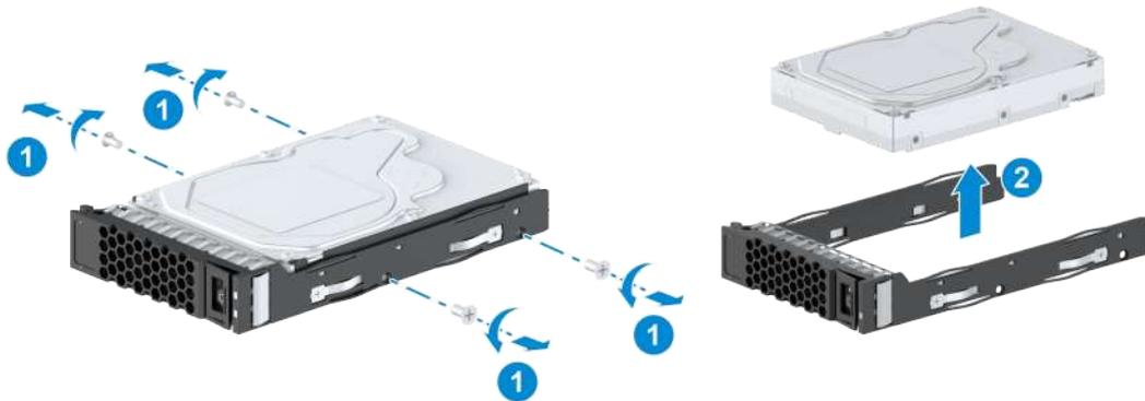
Figure 3-3 Removing a 2.5-Inch Hard Disk
