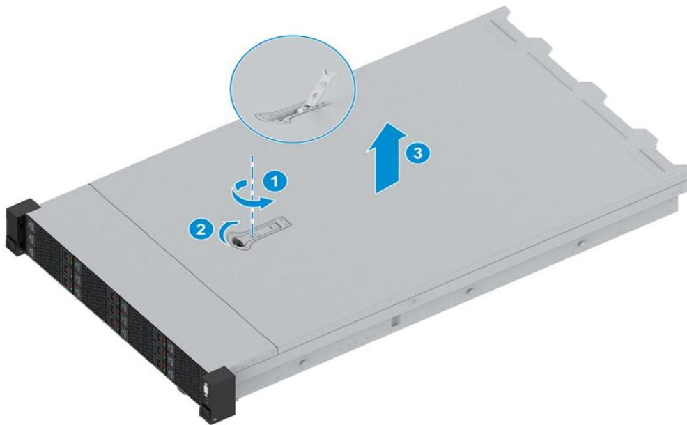
3. Open the ejector lever of the server cover, and push the cover backwards, see ② in [Figure 2-11](#).
