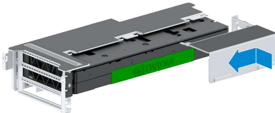
6. Tighten the fastening screws of the GPU support bracket by using a PH2 crosshead screwdriver, see [Figure 3-56](#).
