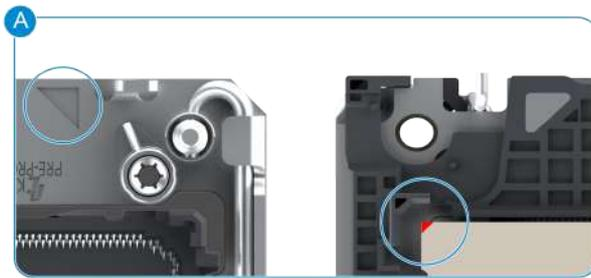
8. Pull the anti-tilt latches in the following directions to lock the heat sink, see [Figure 3-90](#).
