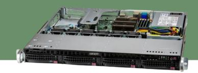
Single Socket H5 (LGA-1200) Intel® Xeon® E-2300 series Processors and 10th Gen. Pentium® Processors
